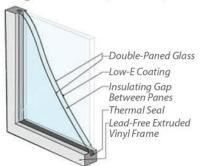
Not only do our super-efficient windows help to keep your energy costs and usage down, the double-paned, insulated, Low-E glass, also helps to protect your new finishes and your furniture from the sun's harmful UV rays, which can cause fading and degradation to textile products. The vinyl window frames substantially reduce heat and cold transfer, and help to prevent moisture accumulation and sweating during seasonal temperature changes.
