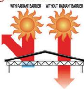
First Texas Homes' standard radiant barrier roof decking can prevent up to 97% of the Sun's radiant heat from entering your attic space. This can result in attic temperature reductions of up to 30 degrees. Because your A/C equipment and ductwork stay cooler, it's easier, and less costly, to maintain comfortable temperatures in your new home.
